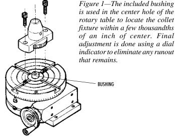
necessary to mount it at an angle across the two T-slots to accommodate the difference between the centerline of the T-slots and hold-down screws.
