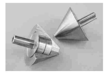
The bullnose live center on the left is cut away to show the two preloaded internal bearings.
