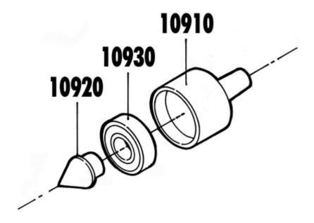
Note: The bearing and nose piece are pressed in at the factory. Once assembled, the 1191 Live Center is not considered user-serviceable. Parts are shown for reference only.
