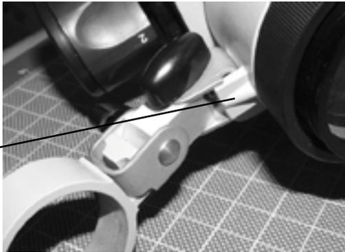
**FIGURE 1**—Shown here is the prototype for the light pivot. The final production versions have a radiused end rather than beveled corners. This solid mount gives a more secure mounting for the light than the one included with the lathe, but it is your option to install it or not.
