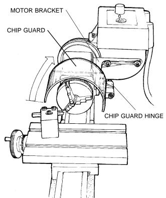
FIGURE 1—The chip guard mounted on a Sherline lathe. The guard pivots up out of the way for access to the spindle area.
