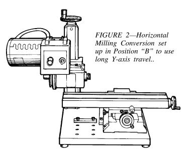
The advantage of this set up is you have 9" of throw from the spindle nose and you could drill and bore a hole 8" from the clamped down edge. If the mill was in its vertical configuration the same edge would interfere with the column. A point to consider is that any axis that moves the work in and out from the end of the spindle becomes the Zaxis and the up and down of the column will usually be called the Y-axis when the mill is in a horizontal configuration.
