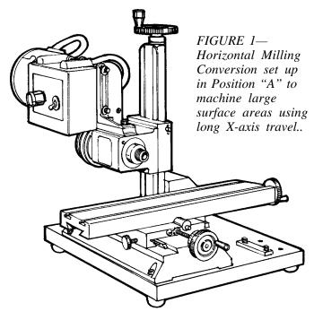
The closest position is used for milling. The configuration of the work has a lot to do with the choice to be made, but remember when milling, the closer the end mills are mounted to the spindle bearings, the more rigid the set up. The spindle can also be mounted lined up with the X-axis by reversing the "XY" table on the horizontal base and mounting the column in the single set of holes.
