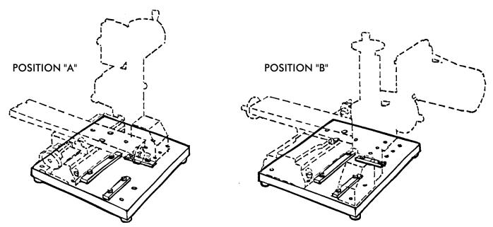
FIGURE 3—Shows suggested position of Mill and alignment bars mounted to Milling Conversion Table for each position. Note that in Position "A", the vertical column and drive can also be mounted further toward the back of the table should your set-up require it.
