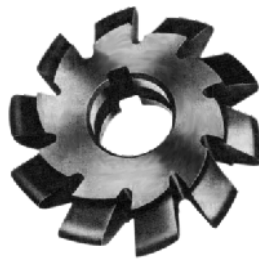
FIGURE 15--A 14-1/2° HSS involute gear cutter
