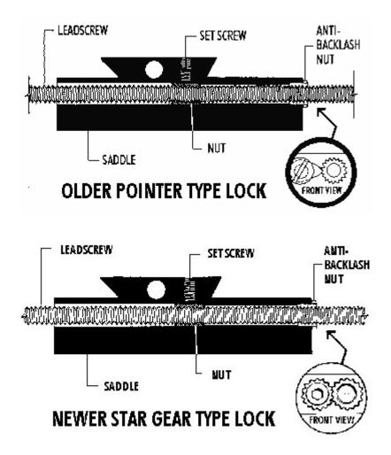
Types of backlash adjustment systems. A new lock now uses a star gear rather than the older style pointer to locate the anti-backlash nut, and a button head socket screw locks it in place. This system is easier to use, but the function is essentially the same. (The hole centers are different, which means the star gear cannot be used to replace the pointer on older models.) The lower drawing shows the older 16-point star gears. The latest system is similar but has more and finer teeth.
