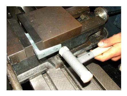
Hold the long leg of the bracket in a bench or mill vise that is fastened down while you tap with a mallet on the short leg to close it up to 90°. Measure with a square to confirm squareness.
