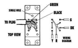
Encoder housing seen from outside with cap removed. Wires are shown in order as they come from the factory. (Click on diagram to view a larger version.)
