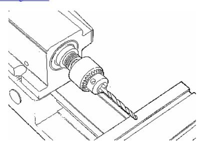
FIGURE 3—Headstock Drilling. The drill turns while the work is held stationary.
