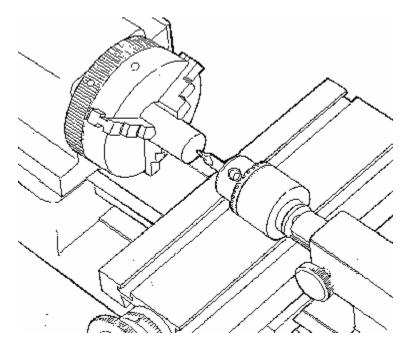
FIGURE 1--Center drilling with a tailstock chuck. The work turns while the drill is stationary.
