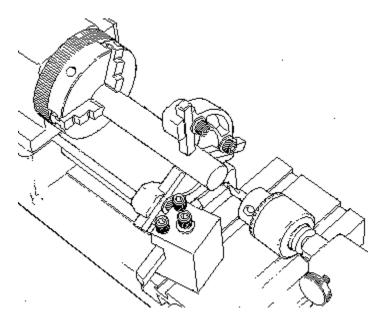
FIGURE 2--Center drilling a long workpiece held in a steady rest.
