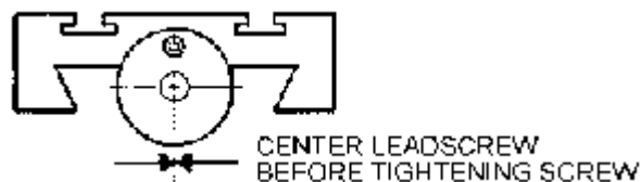
FIGURE 2-Making sure the leadscrew is centered
