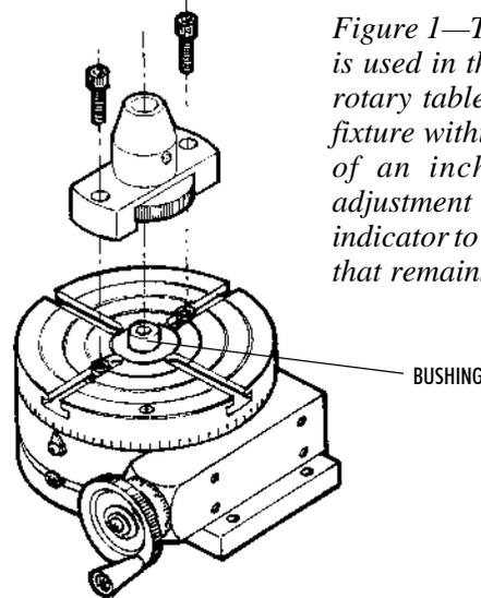
Figure 1—The included bushing is used in the center hole of the rotary table to locate the collet fixture within a few thousandths of an inch of center. Final adjustment is done using a dial indicator to eliminate any runout that remains.
