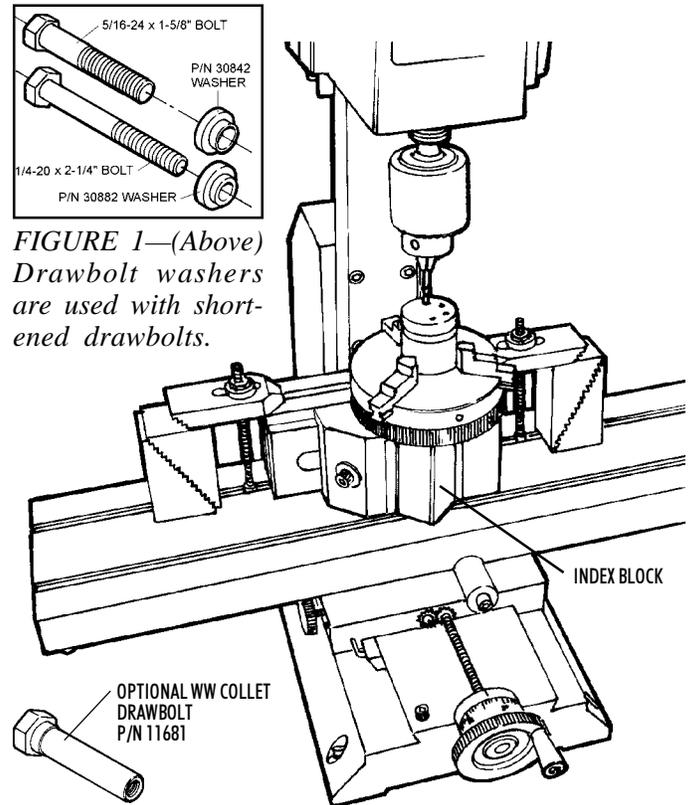
FIGURE 1—(Above) Drawbolt washers are used with shortened drawbolts.
