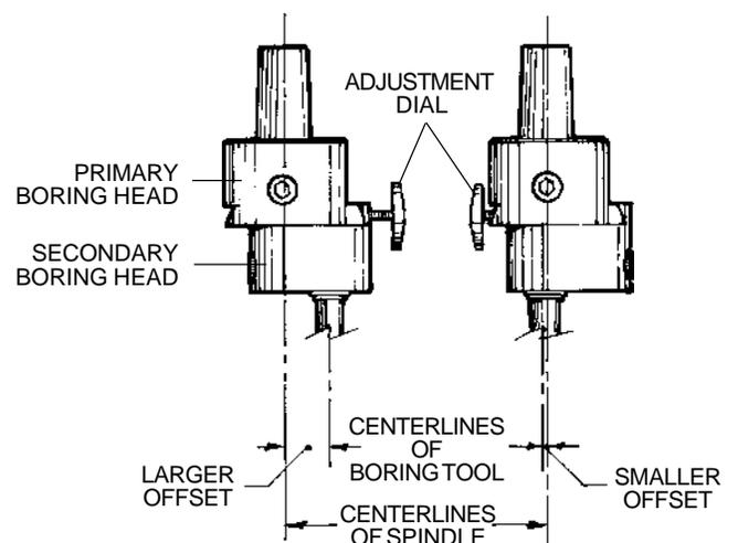
Clamp the boring tool into the boring head so the cutting face of the tool is in alignment with the center of the spindle.
