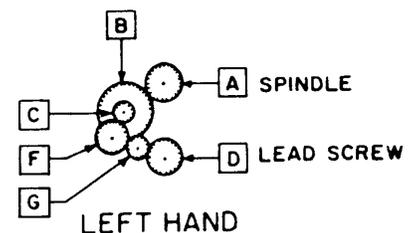
NOTE—Gear "E" or "F" and "G" are idler gears and are used to transmit power and control direction of rotation only. See drawings on page 7 for more detail of how gears are actually installed on the support arms.
