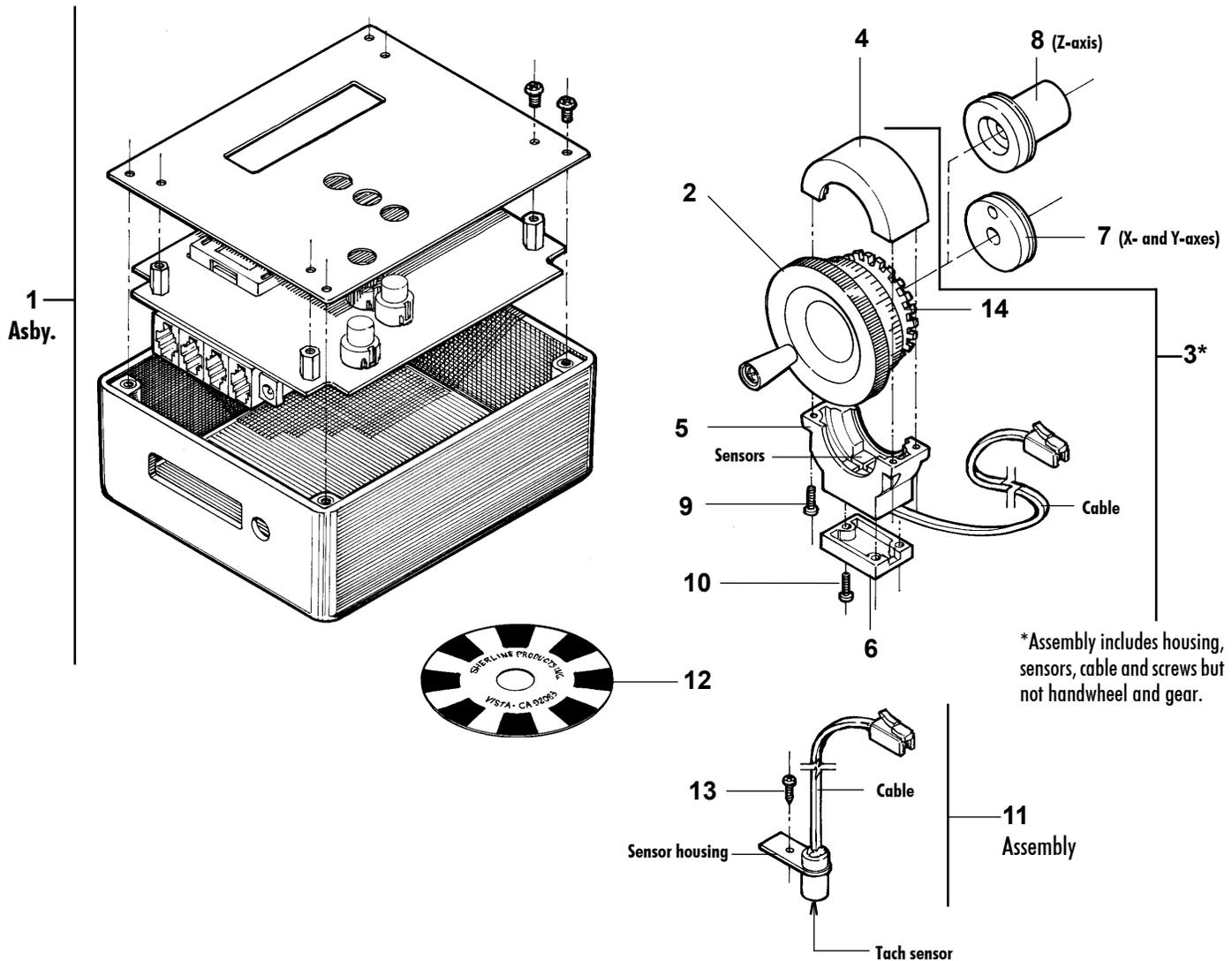
\*Assembly includes housing, sensors, cable and screws but not handwheel and gear.
