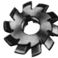
FIGURE 15—A 14-1/2° HSS involute gear cutter
