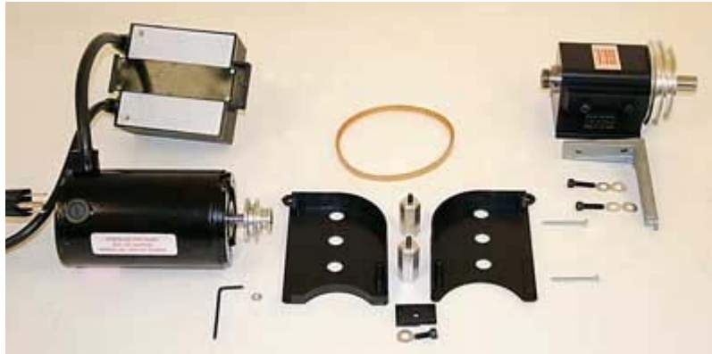
FIGURE 3—Gather all the components. The motor bracket, drive belt and motor mounting screws are in one parts bag, the belt guard, standoffs and screws are in another. The motor bracket screws come threaded into their holes in the headstock. (Click on photo for larger image. This also applies to all the photos below.)
